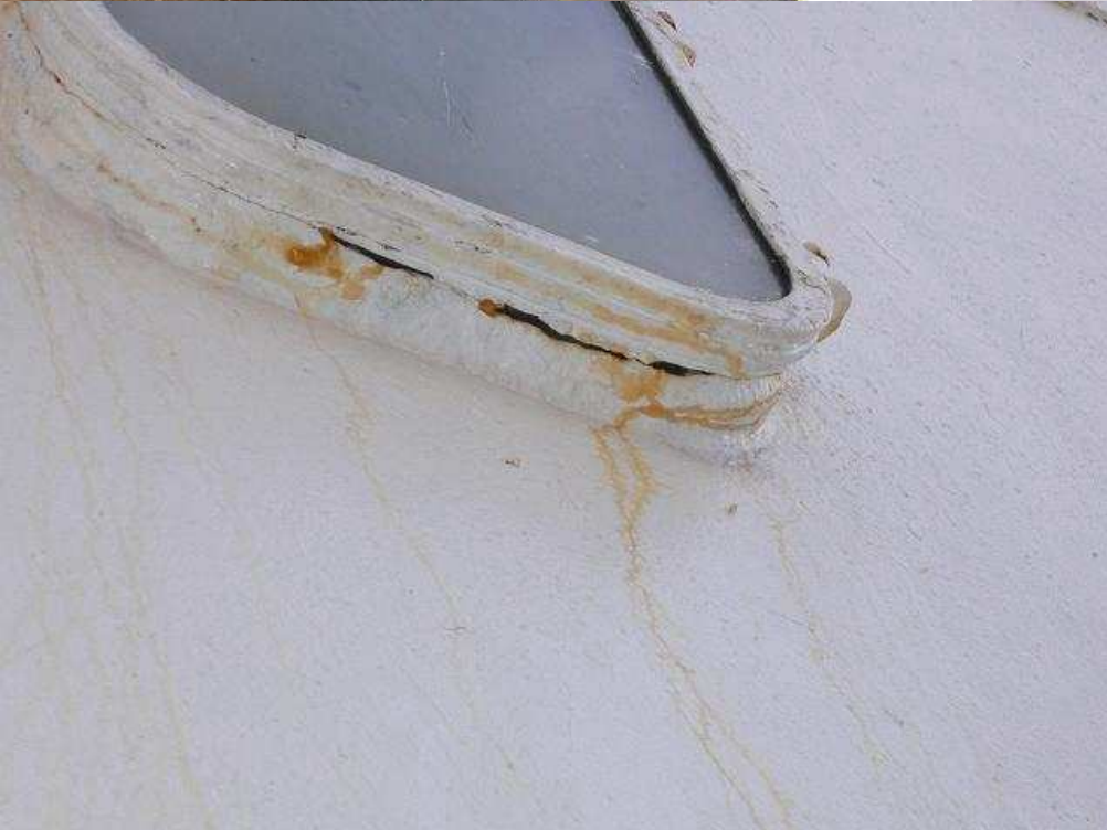
MV Iran Amanat: Poor maintenance of fire dampers and windows
